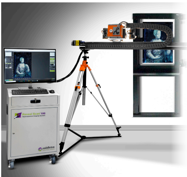
Figure 3. RevealScan 100 Hyperspectral Imaging System for art and cultural heritage from Middleton Spectral Vision.
