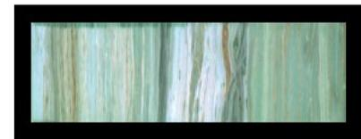
The Green River oil shale sample is a highly laminated mudrock with substantial lamina-scale mineralogical variability, as illustrated by the HSI and micro-XRF results. Multiple mineral components are distinguished by chemometric (MCR) analysis (right).
