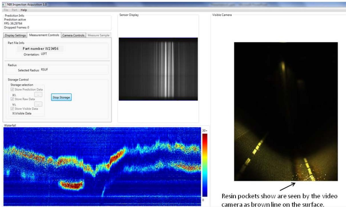
Figure 6 Data collection and live-display software. This image shows a series of surface resin pockets in the NIR image and a visible resin feature on the surface in the video image.
