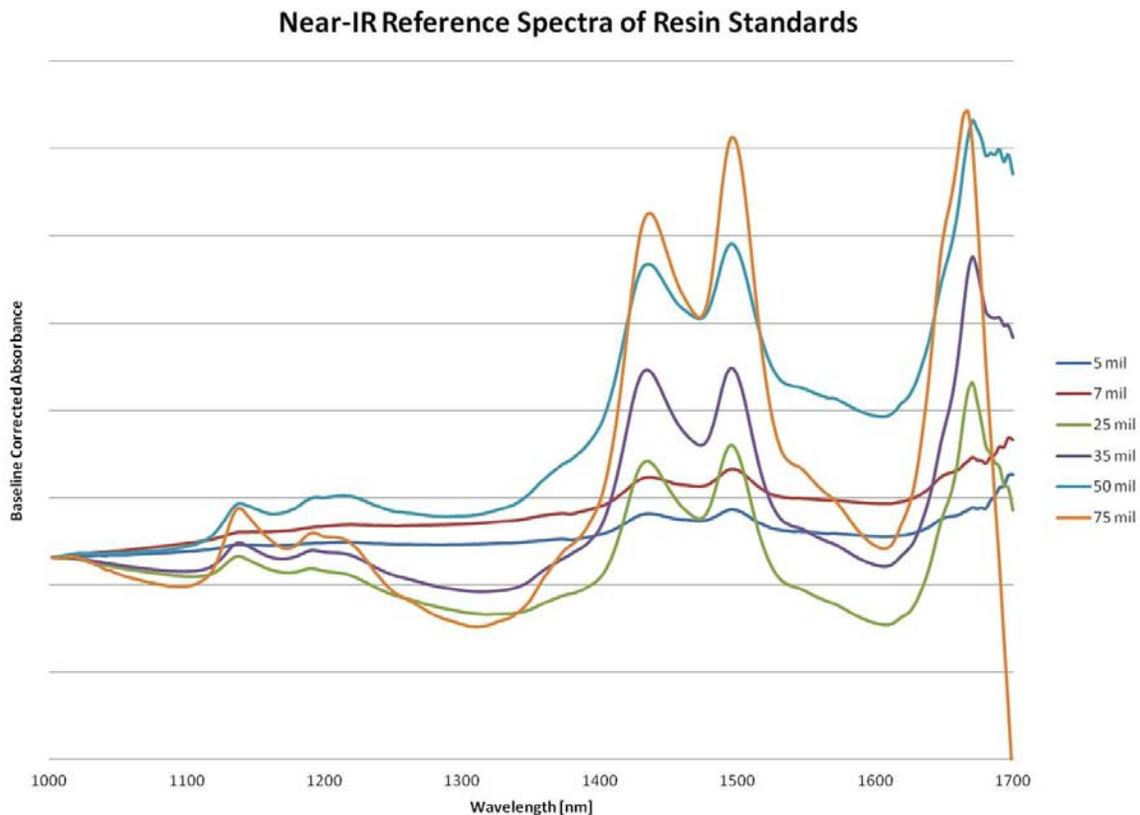
Figure 3 Near infrared spectra (1000 to 1700 nanometer range) for a range of epoxy resin thickness standards (spectra were normalized at 1000 nm for comparison).
