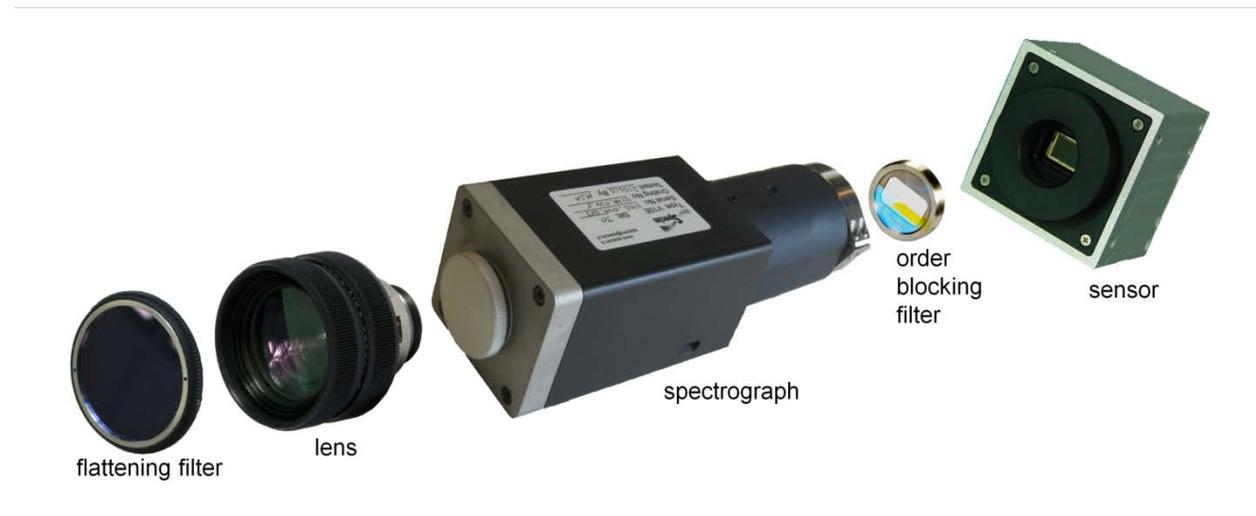
Figure 1 Simplified push-broom hyperspectral camera components diagram.
