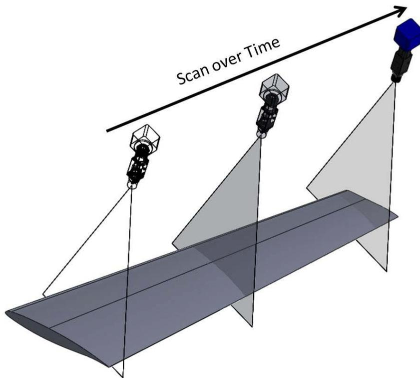
Figure 2 Diagram of the hyperspectral camera scanning over the exterior of a part.
