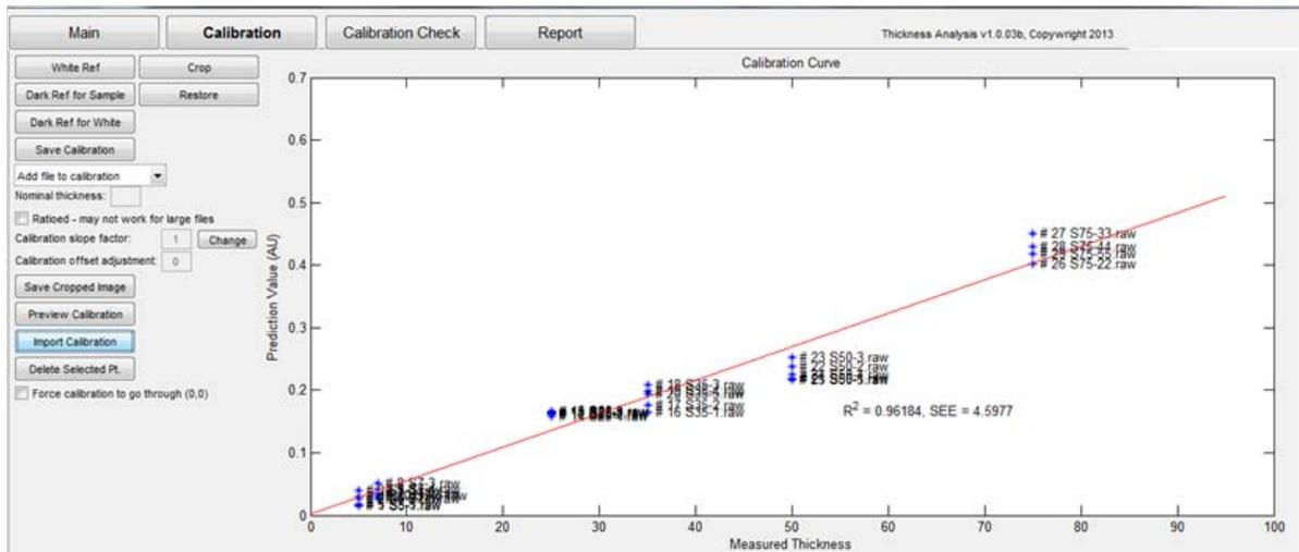
Figure 5 Example resin thickness calibration in the Thickness software.
