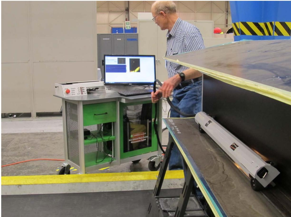
Figure 4 Operator running the NIR measurement on one of the outer radii on a composite test article.
